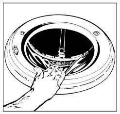
Check the folds in the door seal for any small articles such as buttons which might be lodged there.
